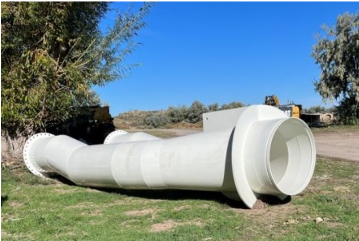
Portneuf Pumping Plant at Fort Hall Indian Irrigation Project, Idaho – prefabricated bifurcation wye.
