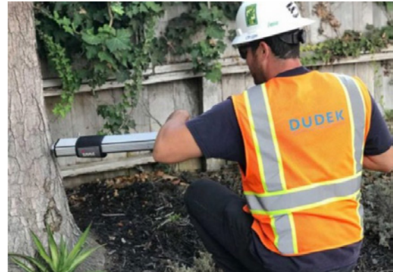
Urban Forester using a LaCroix Resistograph tool on a tree to detect decay in the wood.
